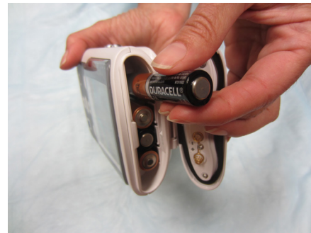
Put in new batteries from the bottom up. Match up the (+) and (-) markings.
