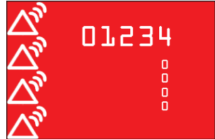
System fault alarm (red) with error code
