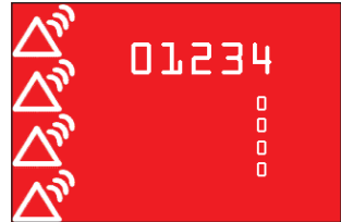
System fault alarm (red) with error code
